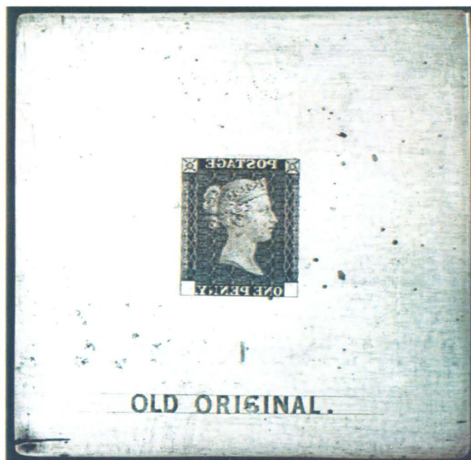
"Old Original" die, complete bar corner letters
