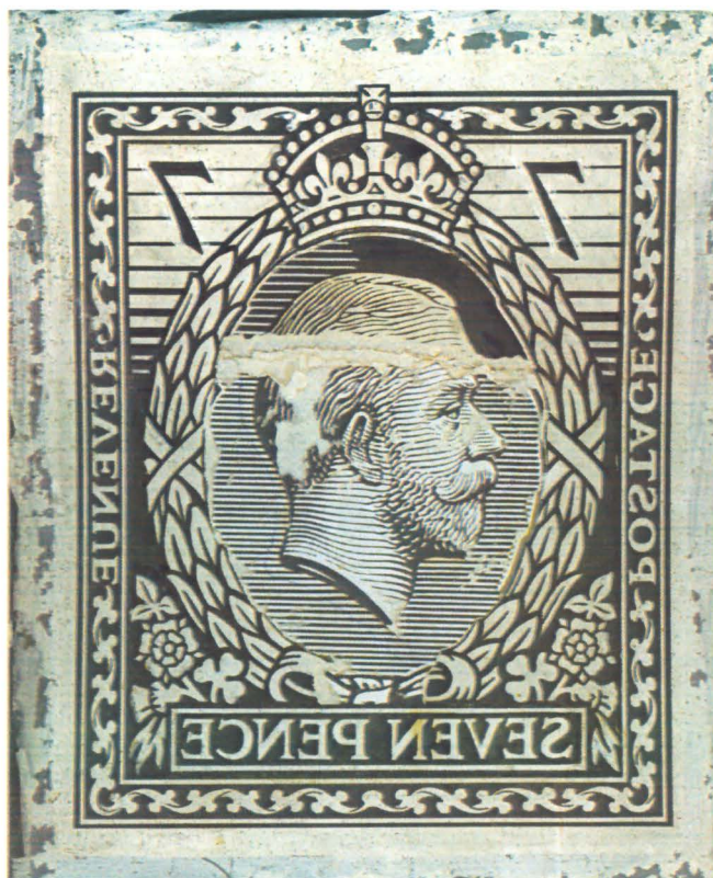
Engraver's drawing (on metal) in reverse for a letterpress stamp
