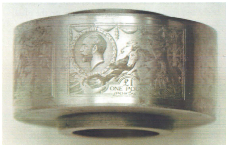
Transfer roller for the Seahorses £ 1 design
