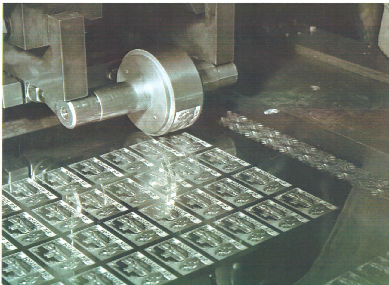
Below: transfer roller rocking the image of the Castles 2/6d to create the plate
